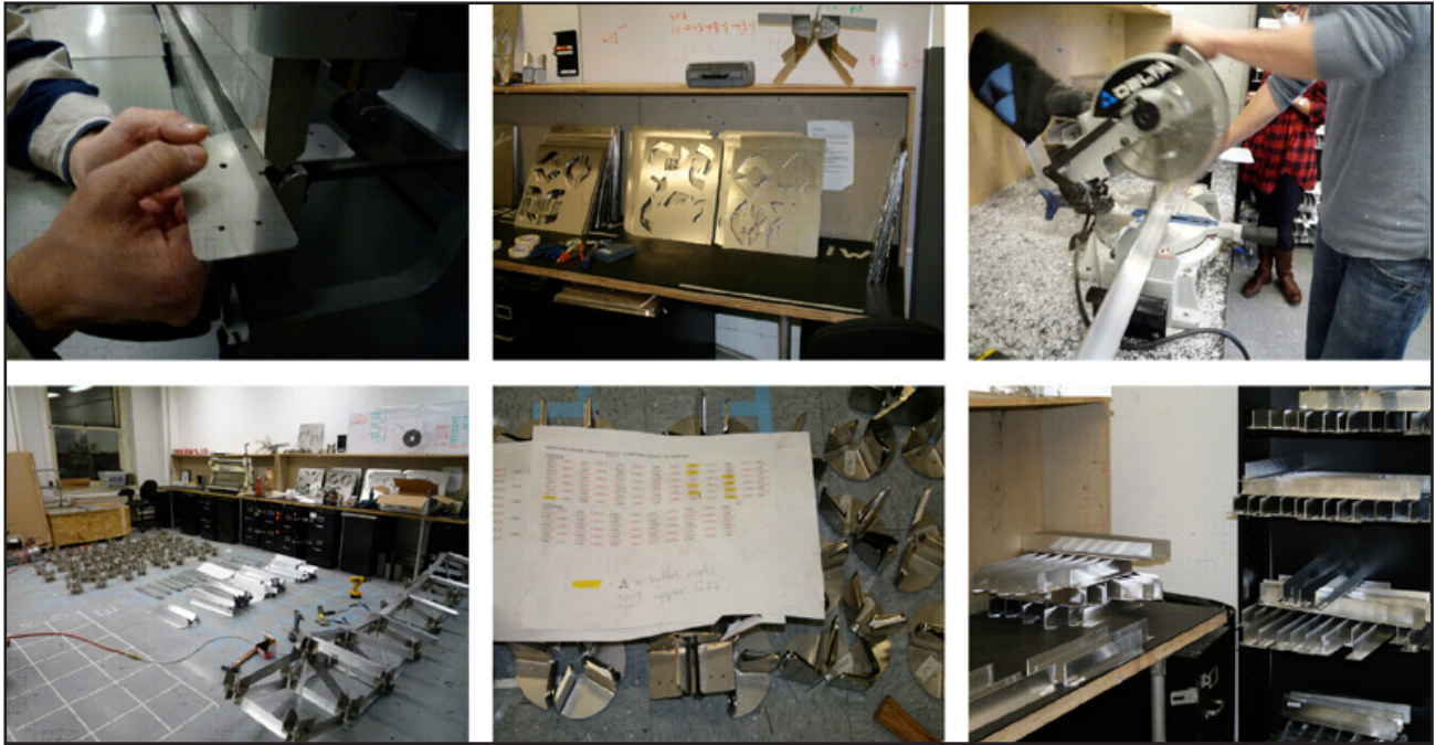
Fig. 5: A combination of digital (laser cut at Maloya Laser) and analogue (cutting structural aluminum extrusions) fabrication techniques were used to produce the nodes and struts; a majority of the production was done at the GSAPP
